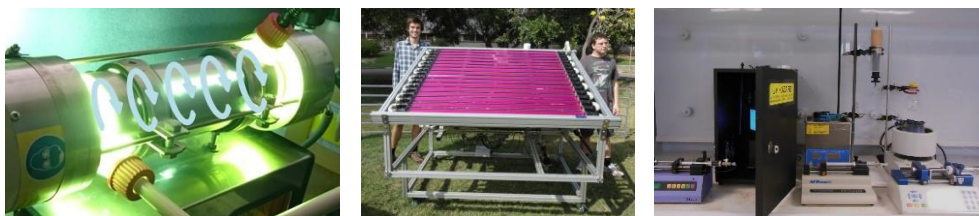
Figure 1. Loop reactor, solar CPC-reactor and photochemical-thermal tandem flow-reactor.
